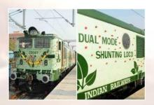
West Central Railway has developed a battery operated dual-mode locomotive named Navdoot. This engine runs on both the modes i.e. battery and electricity. Presently it is being used during shunting of trains at Jabalpur, Mudwara and other stations on trial basis. This dual mode locomotive has also received the Best Innovation Award from the Railway Board. With this new locomotive, Railways will save 1000 liters of diesel per day. It will be used more after clearing all the trials.
